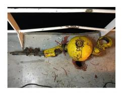
Headache ball and hook assembly on deck after impact.
